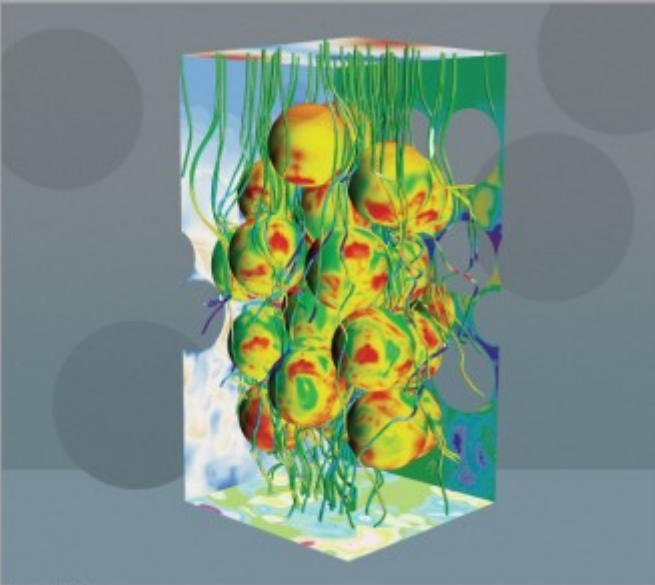
Flow through randomly stacked nuclear pebbles
